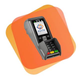
The V200c is characterized especially by compact dimensions. Combined with the integrated highperformance printer, the V200c is ideal for small- and medium-sized businesses. The strong performance of the Cortex A9 processor enables ideal performance for a smooth transaction process. The contactless reader, which is placed at the height of the display, supports NFC-enabled smartphones as well as smartwatches in addition to contactless-enabled cards.
