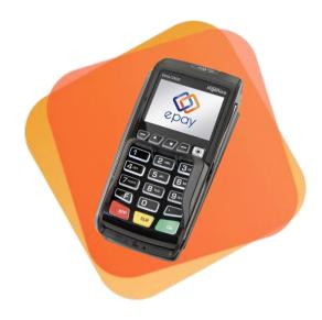
With its large, high-resolution display and simple keyboard layout, the Ingenico Desk 3500 is easy to use. The contactless reader, which is located above the display, supports all contactless-capable cards as well as NFC-capable smartphones and smartwatches. The checkout area stays tidv thanks to the which communication box. is separated by a cable.
